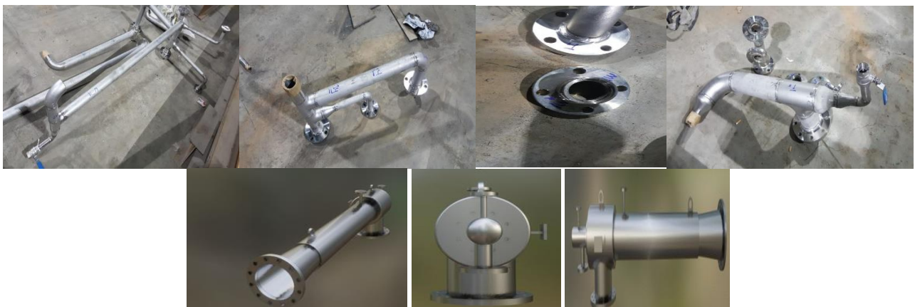
Figure 5. The ejector's manufacture and assembly
