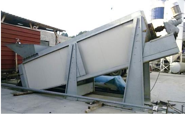
Figure 14. Prototype of an auger drier of the Personal Factory
