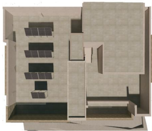
Figure 13. Roof PV panels distribution
