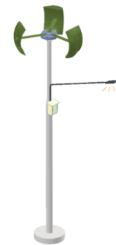
Figure 10. Illustration of stand-alone street lighting by a small vertical axis wind turbine using the axial generator
