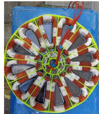
Figure 4. Axial generator wire winding of stator topology
