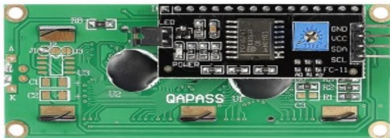
Figure 11. LCD with I2C hardware mounted on it
