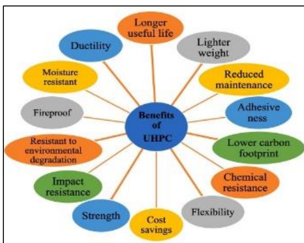
Figure 1. Significant benefits and properties of UHPC [1]
