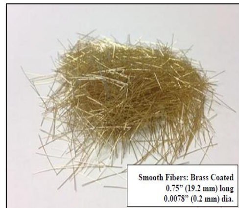
Figure 3. Sample of Steel Fibers (utilized as 1.5% in UHPC) [53]
