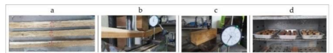
Figure 7. Testing of the a) fracture coefficient; MOR (ksc.), b) coefficient of elasticity; MOE (ksc.), c) wood hardness (kg.), and d) moisture content (%)*
