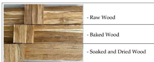
Figure 6. The changes of the teak wood from the process of baking, soaking, and drying
