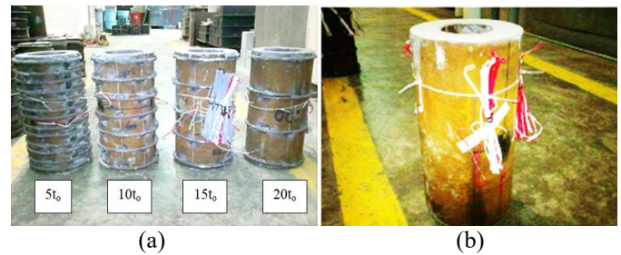
Figure 1. CFDST Columns: (a) Without External Steel Ring and (b) With External Steel Rings ( s=5to, 10to, 15to and 20to ) [46]
