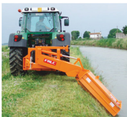
Figure 14: Examples of implements belonging to scenario/category 2 of Table 1; (left) lateral shredder [44]; (right) single sickle bar [45].
