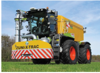
Figure 15: Examples of implements belonging to scenario/category 3 of Table 1; (left) ‘Claas Xerion Saddle Trac’ multi-purpose tractor with slurry tanker equipment on the rear axle [46]; (right) ‘Fendt F 345 GT’ implement carrier with a tipper body on the front axle [47].
