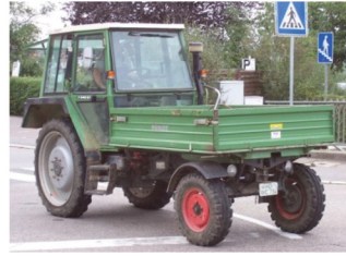
Figure 15: Examples of implements belonging to scenario/category 3 of Table 1; (left) ‘Claas Xerion Saddle Trac’ multi-purpose tractor with slurry tanker equipment on the rear axle [46]; (right) ‘Fendt F 345 GT’ implement carrier with a tipper body on the front axle [47].
