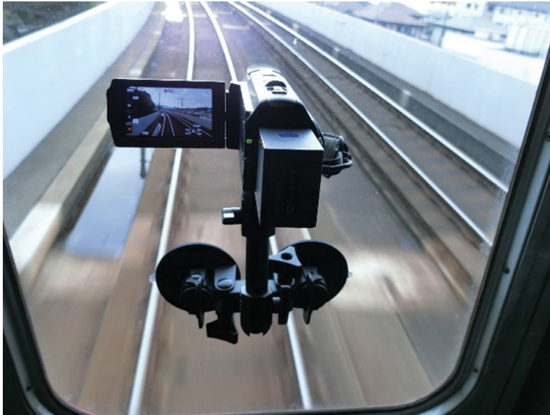
Figure 1: Shooting a video sequences on the front of commercial train ( source: Nagamine et al., 2020 ) [5].
