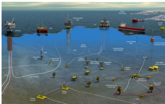
Figure 1: Subsea processing system (Seadiscovery.com).
