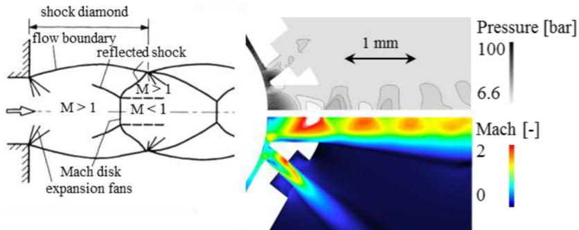
Figure 1: Theory (left): Rotationally symmetric underexpanded high-pressure free gas jet [9]. Simulation (right): Pressure and velocity profile of gas jet emerging from injector A for top dead centre conditions.  $p_{\text{Rail}} = 100$  bar,  $p_{\text{Cyl}} = 21.26$  bar,  $T_{\text{Air}} = 750$  K,  $t = 1$  ms after SOI (CFX,  $10 \mu\text{m}$  mesh spacing).
