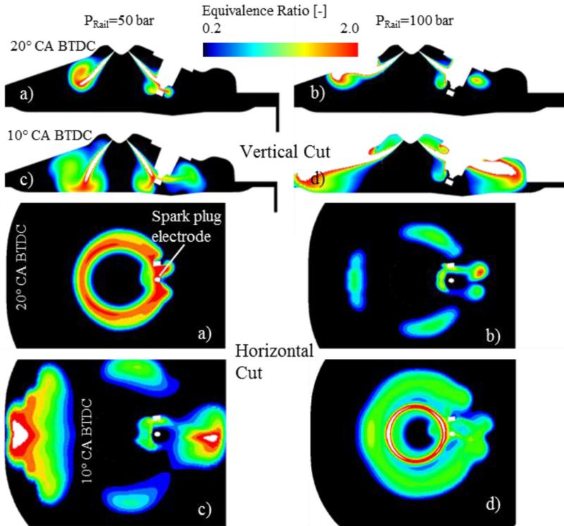
Figure 8: Mixture formation with Injector B for two different rail pressures and times:  $p_{\text{Rail}} = 50$  bar (a) & (c) and  $p_{\text{Rail}} = 100$  bar (b) & (d);  $t = 20^\circ$  CA BTDC (a) & (b) and  $t = 10^\circ$  CA BTDC (c) & (d). Performed on a mesh with 13.1 million cells.
