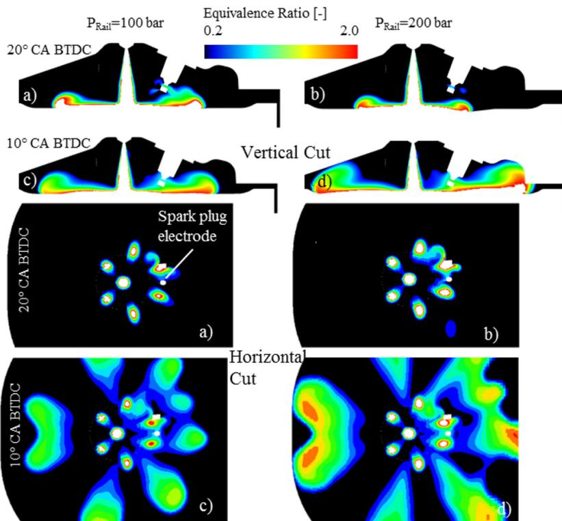
Figure 6: Mixture formation with Injector A for two different rail pressures and times:  $p_{\text{Rail}} = 100$  bar (a) & (c) and  $p_{\text{Rail}} = 200$  bar (b) & (d);  $t = 20^\circ$  CA BTDC (a) & (b) and  $t = 10^\circ$  CA BTDC (c) & (d). Performed on mesh with 13.5 million cells.
