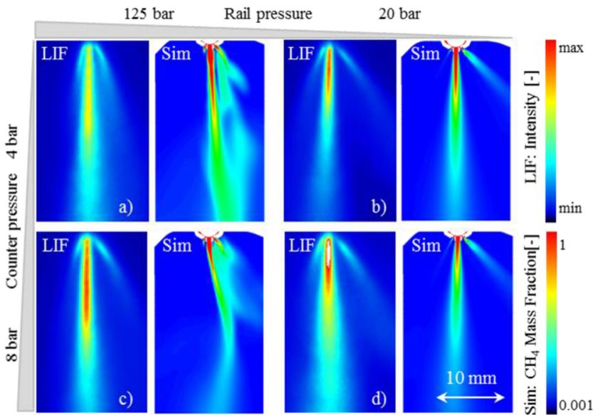
Figure 3: Gas jet from injector A at  $t = 2$  ms after SOI (a) + (b) air density  $\rho_{\text{Air}} = 3.3 \text{ kg/m}^3$  (c) + (d)  $\rho_{\text{Air}} = 5.3 \text{ kg/m}^3$ . Experimental results from LIF (left) and simulation results using Fire (right), mesh: 1.8 million cells.
