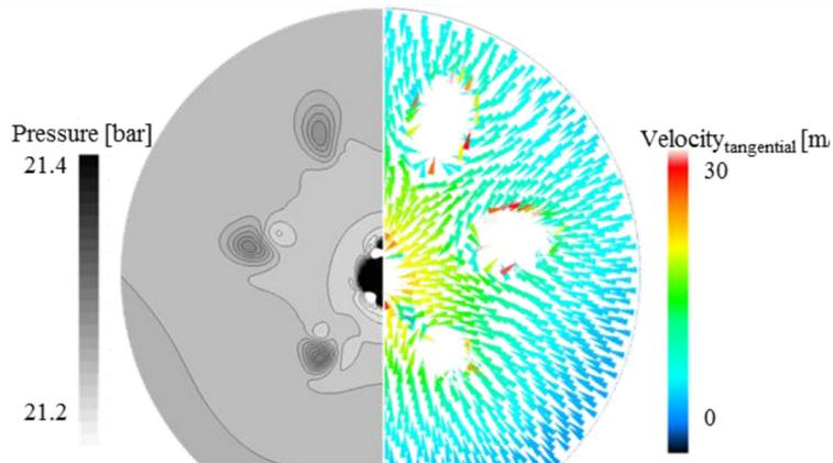
Figure 2: Pressure and tangential velocity on horizontal cut 1 mm downstream the nozzle orifice (Injector A) for top dead centre conditions.  $p_{\text{Rail}} = 100$  bar,  $p_{\text{Cyl}} = 21.26$  bar,  $T_{\text{Air}} = 750$  K,  $t = 1$  ms after SOI (CFX,  $10 \mu\text{m}$  mesh spacing).
