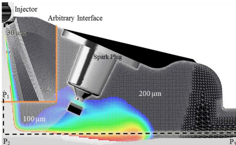
Figure 5: Refinement levels of the mesh (13.5 million cells) used for the in-cylinder calculations.
