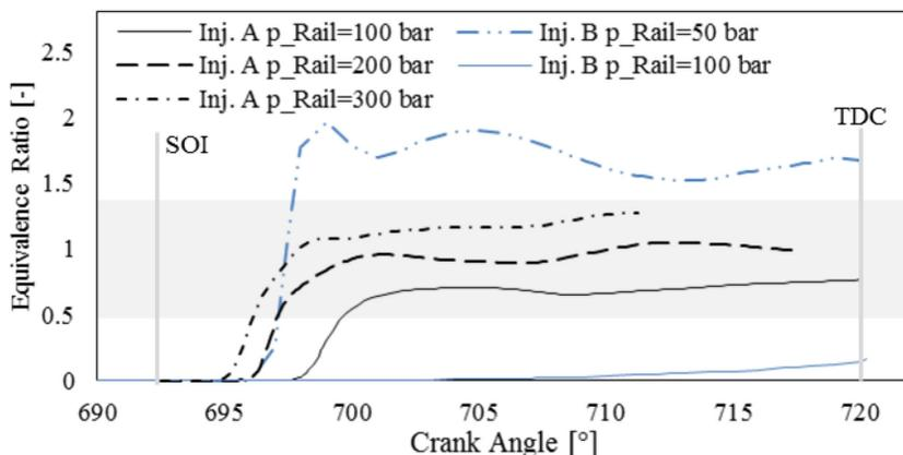
Figure 7: Equivalence ratio at the spark plug for Injectors A and B for different rail pressures.
