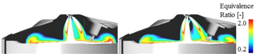
Figure 4: Jet behaviour emerging from injector A for increasing mesh resolution: 4.5 million cells (left) and 23.6 million cells (right). Conditions at top dead centre  $p_{\text{Rail}} = 100$  bar,  $p_{\text{Cyl}} = 21.26$  bar,  $T_{\text{Air}} = 750$  K,  $t = 1.8$  ms after SOI (CFX).
