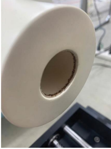
Figure 10. The sandpaper stripe attached to the inner surface of the nozzle near the exit
