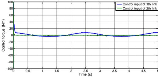
**Figure 9.** Control torque of both links with initial condition  $[0.2, 0.1]$
