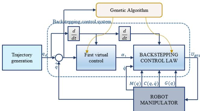
Figure 4. The proposed optimized control scheme
