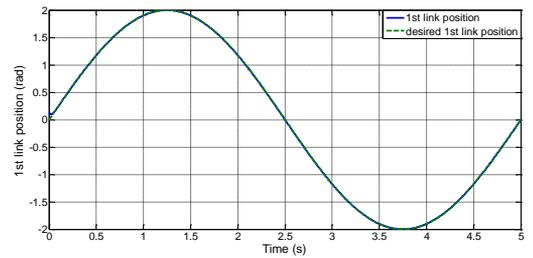
**Figure 12.** First link's  $q_1$  angle position response under the initial condition 0.2 and disturbance  $d$
