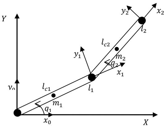
Figure 6. 2-dof robot system
