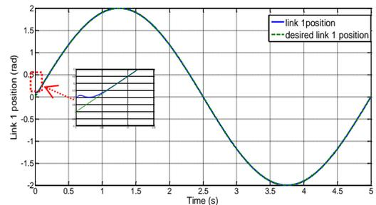
Figure 7. First link's  $q_1$  angle position response under the initial condition 0.2
