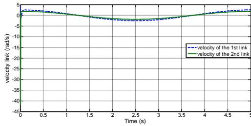
**Figure 15.** Time responses velocity of both links with initial condition  $[0.2, 0.1]$ , and disturbance  $d$
