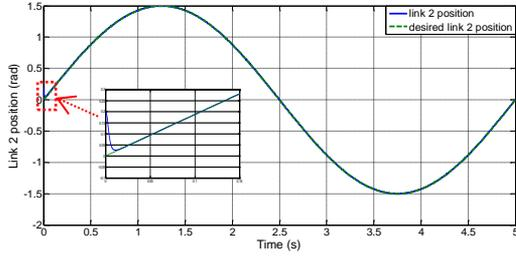
**Figure 8.** Second link's  $q_2$  angle position response under the initial condition 0.1
