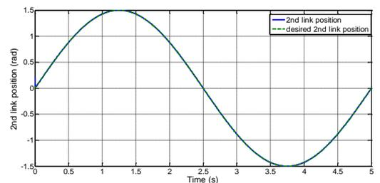
**Figure 13.** Second link's  $q_2$  angle position response under the initial condition 0.1 and disturbance  $d$
