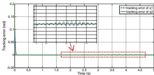
**Figure 16.** Time responses of tracking errors for both links with initial condition  $[0.2, 0.1]$ , and disturbance  $d$
