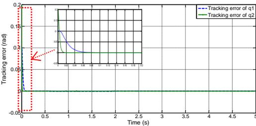
**Figure 11.** Time responses of tracking errors for both links with initial condition  $[0.2, 0.1]$
