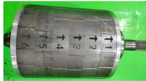
Figure 10. Rotor lamination prototype with six steps of V-skew magnet slices
