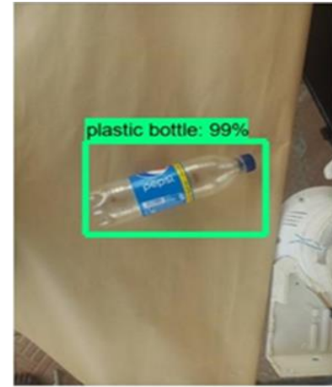
Figure 14. Detection of Pepsi plastic bottle by the TensorFlow object detection model
