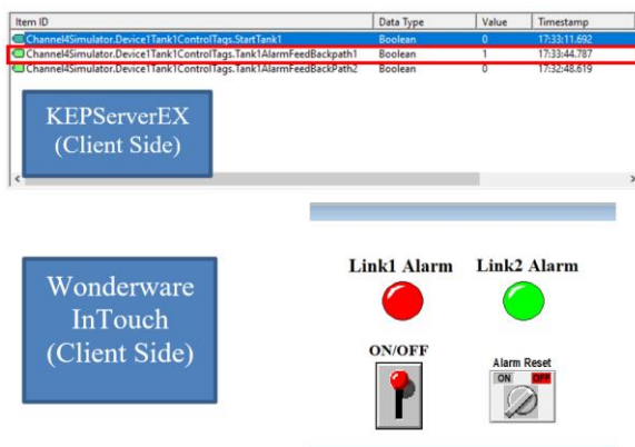
Figure 7. Alarm initiation due to Link1 disconnection between the OPC UA server and the OPC UA client
