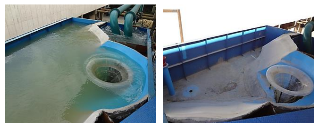
Figure 2. A view of the model built from the morning glory spillway of Haraz dam before and after impounding [12]
