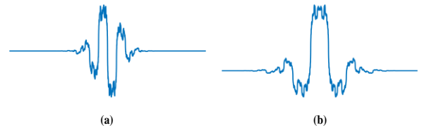
Figure 2. Biorthogonal 3.5 wavelet pair: (a) decomposition and (b) reconstruction wavelets
