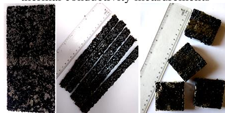
Figure 3. The plate, specimens and the parallelepipeds of elaborated composites
