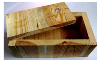
Figure 2. Wood moulds for three-point bending test and thermal conductivity measurements
