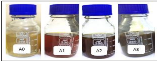
Figure 3. Feature shifts in the color of colloidal solutions which can be Ag-NPs /(CM CS - isopropanol)) after being exposed to (0, 768, 1151, 1920 Gy) doses (A0–A3, respectively)
