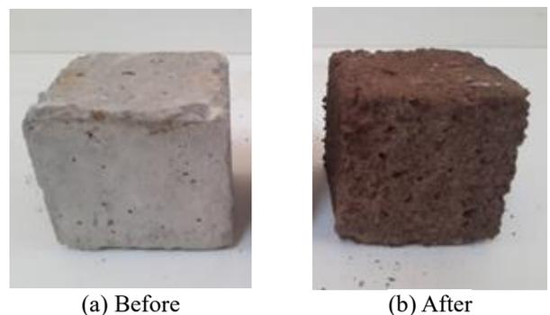
**Figure 12.** Test specimens stored in acid (HCl)
