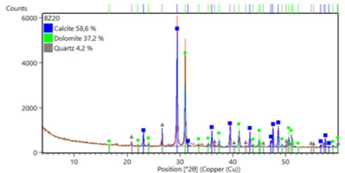
**Figure 3.** X-Ray diffractogram of the pozzolana
