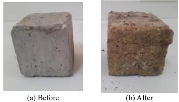
**Figure 11.** Test specimens stored in acid (H<sub>2</sub>SO<sub>4</sub>)
