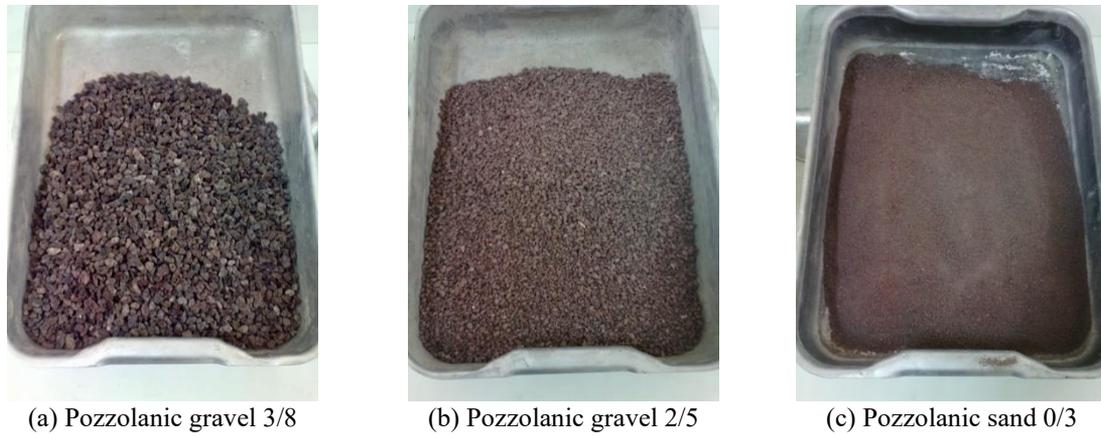
**Figure 1.** Pozzolanic aggregates
