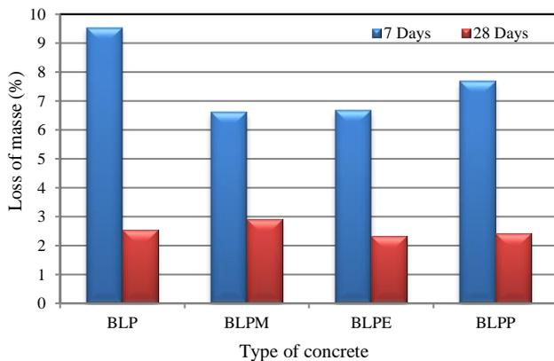
**Figure 9.** Loss of mass of specimens kept in sulfuric acid (H<sub>2</sub>SO<sub>4</sub>) as a function of temperature 200°C
