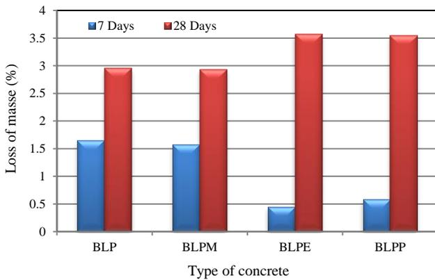
**Figure 8.** Loss of mass of specimens stored in acid (HCl) according to the temperature 600°C
