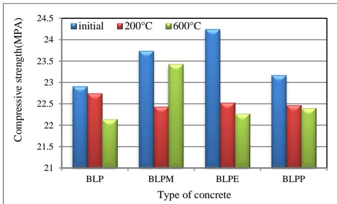
**Figure 15.** Compressive strength of specimens stored in H<sub>2</sub>SO<sub>4</sub> (7 days)
