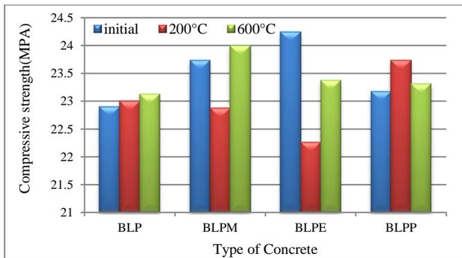
**Figure 14.** Compressive strength of specimens stored in water (28 days)
