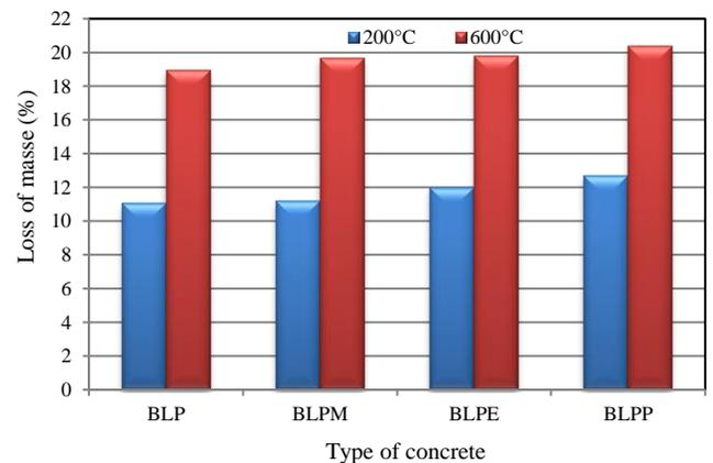
**Figure 6.** Mass loss of specimens after heat treatment
