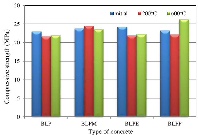
**Figure 17.** Compressive strength of specimens stored in HCl acid at 7 days
