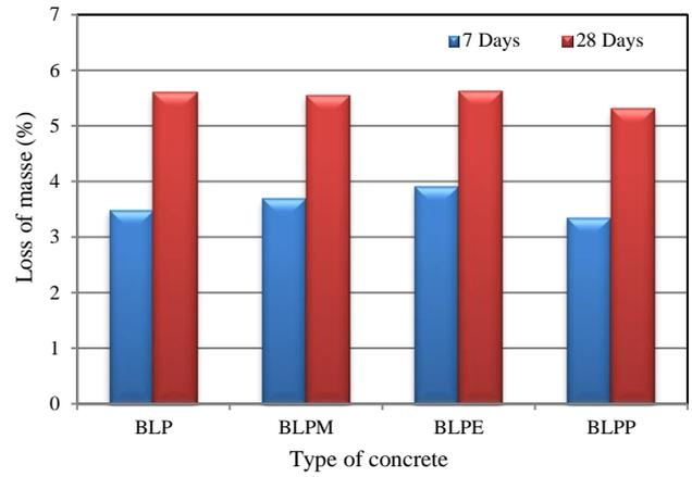
**Figure 10.** Loss of mass of specimens kept in sulfuric acid (H<sub>2</sub>SO<sub>4</sub>) as a function of temperature 600°C
