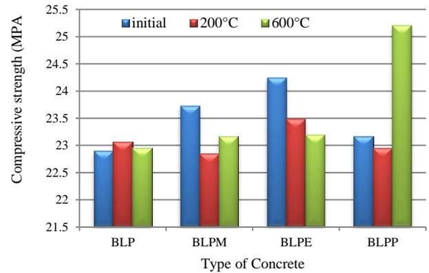
**Figure 16.** Compressive strength of specimens stored in H<sub>2</sub>SO<sub>4</sub> (28 days)
