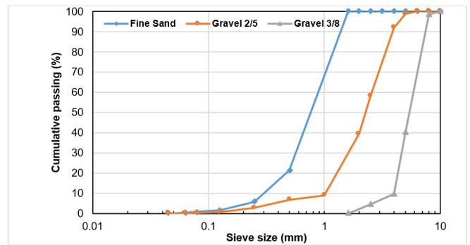
**Figure 2.** Particle size distribution of the different granular fractions
