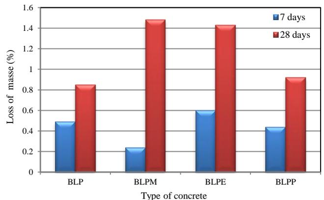
**Figure 7.** Loss of mass of specimens stored in acid (HCl) according to the temperature 200°C
