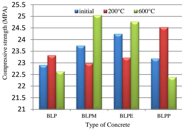
**Figure 13.** Compressive strength of specimens stored in water (7 days)
