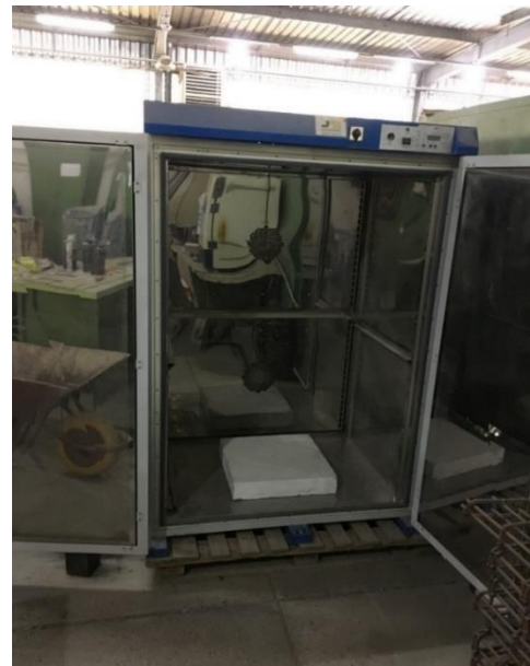
Figure 2. Heating the voided slabs
