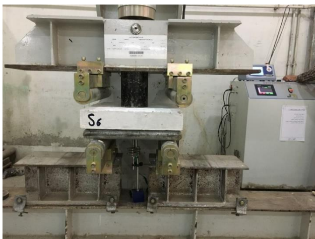
Figure 3. One of the voided slab specimens under testing
