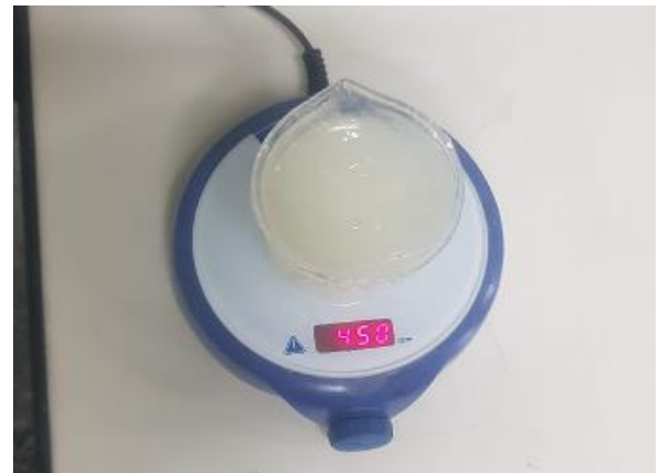
Figure 2. Magnetic stirrer utilizes for mixing nanoparticles into CT232 cutting oil
