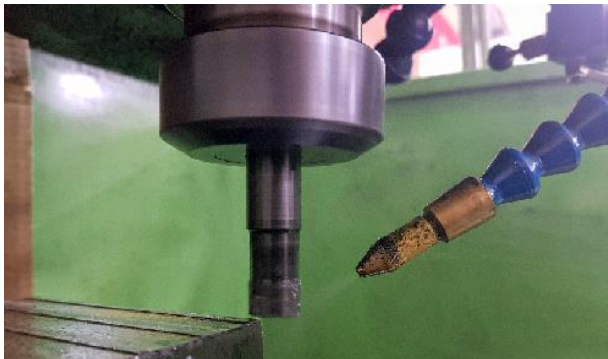
Figure 4. Milling operation running with nanofluid MQL
