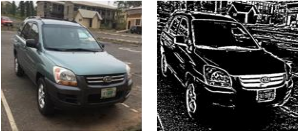
Figure 3. Image binarization using Otsu thresholding
