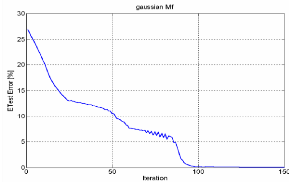
Figure 5. Testing error for ANFIS configuration with Gaussian Mf and Traingular Mf
