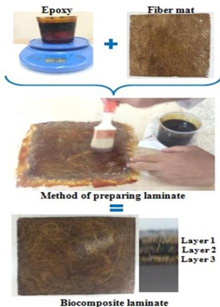
**Figure 5.** Method of preparing biocomposite laminate
