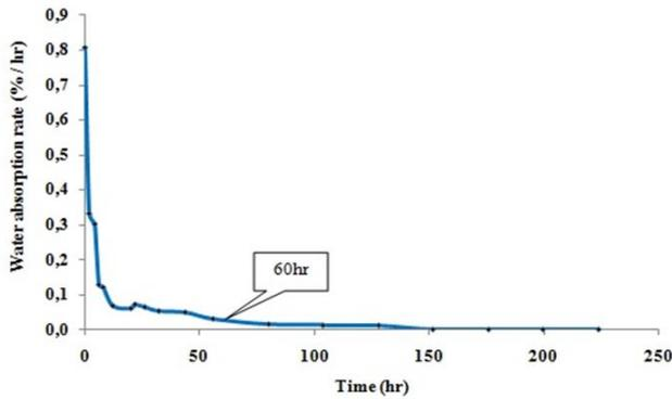
**Figure 10.** The water absorption rate of epoxy composite reinforced with *Lif* fiber mat
