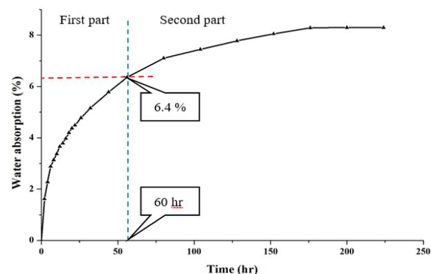
Figure 9. The water absorption of epoxy composite reinforced with *Lif* fiber mat
