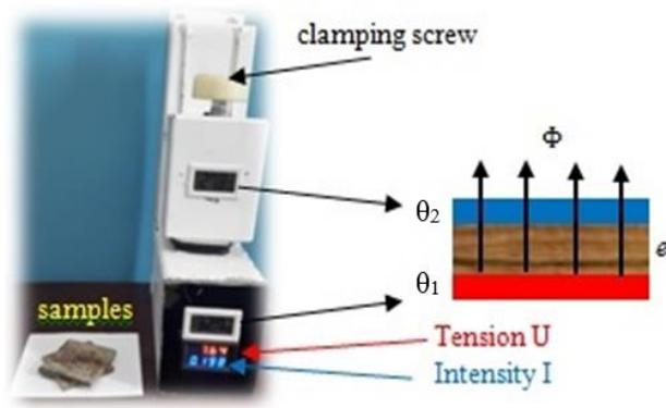
Figure 7. Thermal conductivity device
