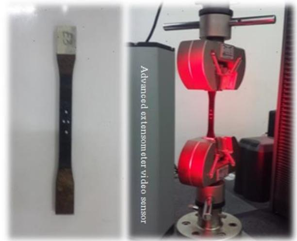
Figure 8. Video-tensile test
