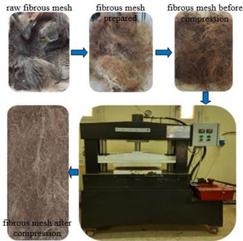
**Figure 3.** Mat fiber preparation protocol
