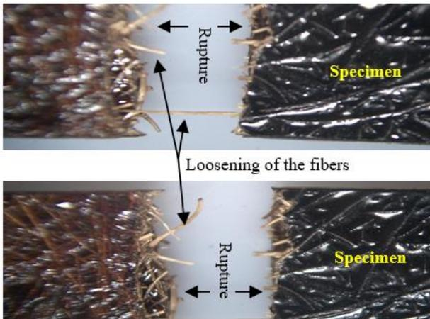
Figure 12. Loosening of the fibers
