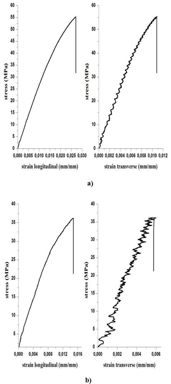
**Figure 11.** Video-tensile test on specimens of a) virgin resin b) composite materials
