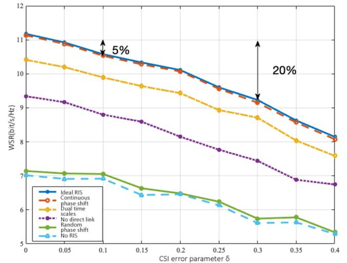
Figure 7. Robustness of joint precoding under CSI errors
