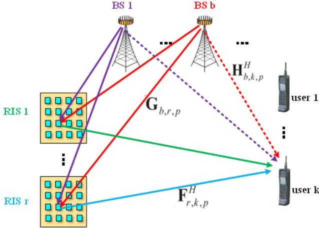
Figure 4. Downlink channel of RIS-CF system
