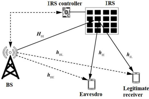
**Figure 2.** RIS-assisted downlink model of MISO
