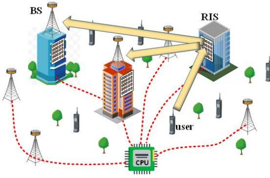
Figure 3. Structure of cellular-free network
