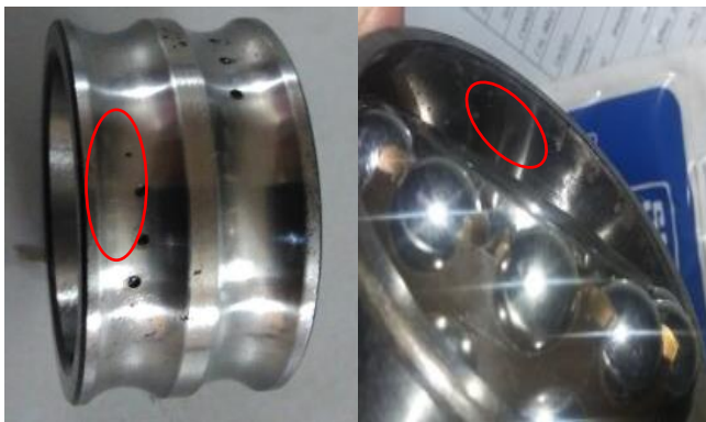
Figure 7. Defects (a) Inner race fault, (b) Outer race fault
