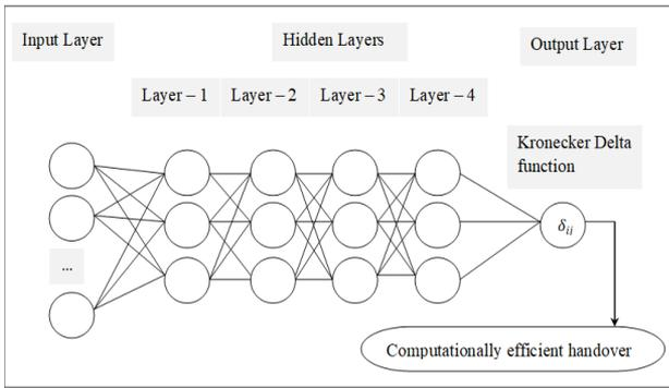
**Figure 3.** Structure of radial Kronecker delta neural network-based optimized handover
