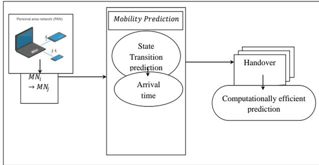
**Figure 2.** Block diagram of Markov renewal prediction-based seamless mobility model
