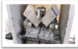
Figure 10. Mode of flexural tensile failure of specimens
