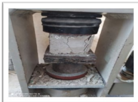
Figure 4. Compression test by crushing used
