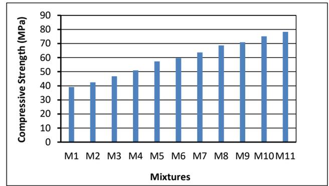
**Figure 4.** Compressive strength of geopolymer at 7 days with 24h curing duration
