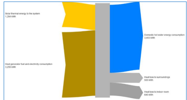
Figure 14. Energy flow diagram of the system when the tilt angle is 40 degrees
