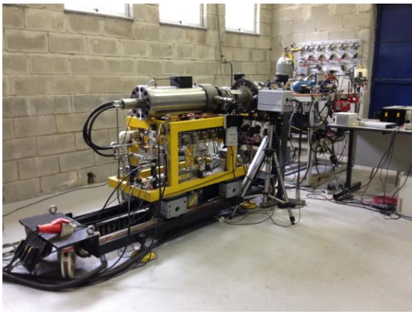
Figure 1. RCM installed on VEL at PUC - Rio
