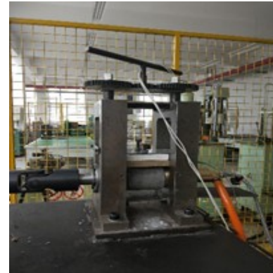
Figure 5. Two-high rolling mill
