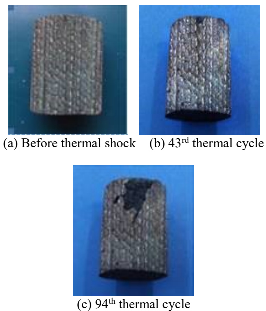
Figure 12. Morphology of laser-remelted samples after thermal shock
