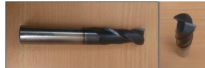
(a) Solid carbide end mill cutter with two flutes
