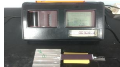
Figure 3. Mitutoyo surfstest SJ-301 surface roughness tester
