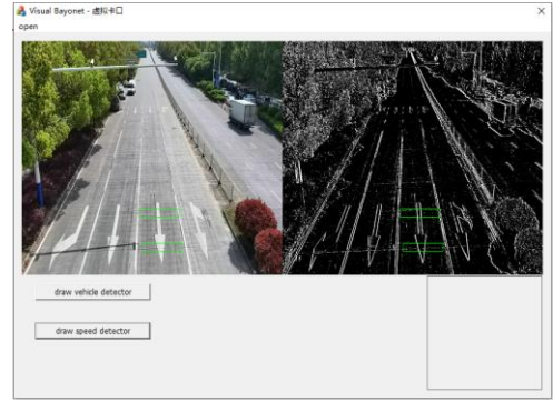
Figure 5. Lane detection coil
