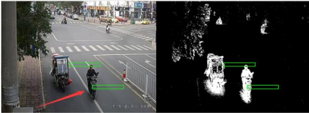
Figure 2. Virtual coil video and its binarization map
