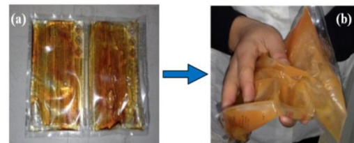
Figure 4. Epoxy resin, (a) before mixing, (b) after mixing
