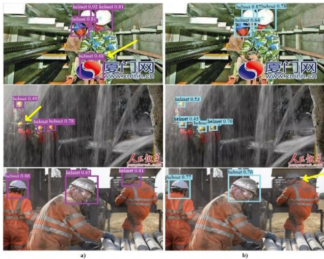
Figure 9. Some failure detection results on the test data with a) ShuffleNetv2, and b) MobileNetv3 as backbone
