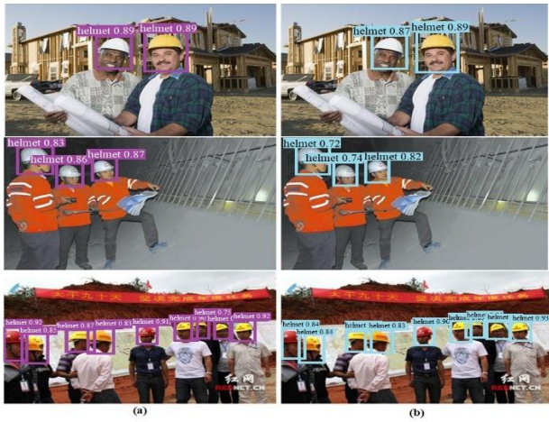
Figure 8. Some true detection results on the test data with a) ShuffleNet v2, and b) MobileNet v3 as backbone
