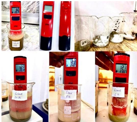
Figure 17. Measure the pH to determine the optimum percentage of Lime
