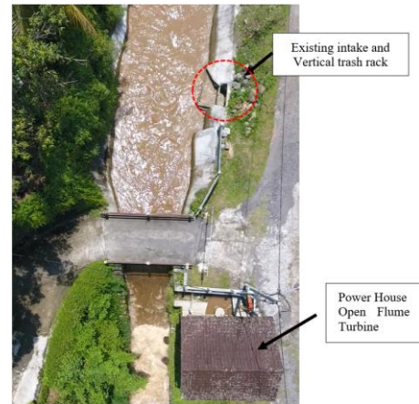
Figure 5. Research location on existing lateral intake and trash rack (Aerial photo of DJI Phantom 4 UAV)
