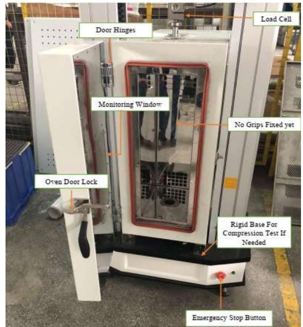
**Figure 2.** Initial oven fitting into the load frame
