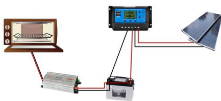
Figure 1. Microwave convective drying system integrated PV system
