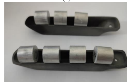
Figure 2. Pre and post de-formation of an upset preform
