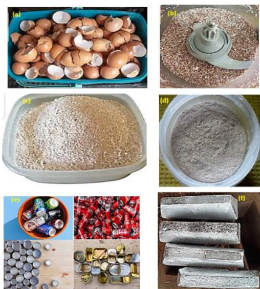
Figure 1. (a) Raw eggshell (b) Pulverized eggshell (c) Milled eggshell (d) Sieved carbonized eggshell (e) Sourced aluminum cans (f) Unreinforced samples casted
