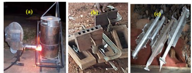
Figure 2. (a) Furnace (b) Cylindrical and rectangular mould (c) Eggshell reinforced casted aluminium
