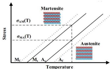
**Figure 1.** The Austenite-Martensite transformations in shape memory alloys
