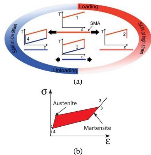
**Figure 2.** (a) Trend of the SMA temperature as a function of strain  $\epsilon$  in the four-stage cycle; (b) corresponding stress-strain diagram
