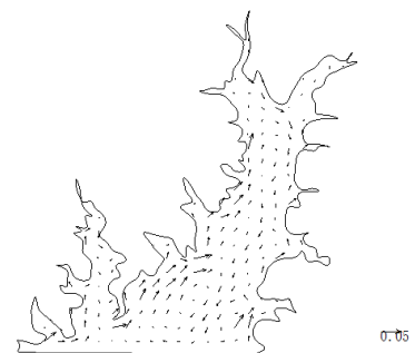
Figure 6. Flow field distribution under 2.7m/s SE wind
