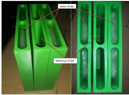
Figure 3. Setup PCM material in the gab sample
