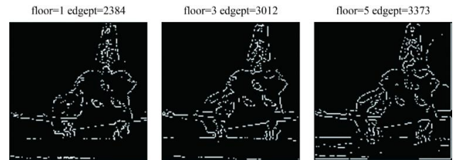
Figure 9. Edge detection results of the 1st, 3rd and 5th layer using Rbio3.1 wavelet
