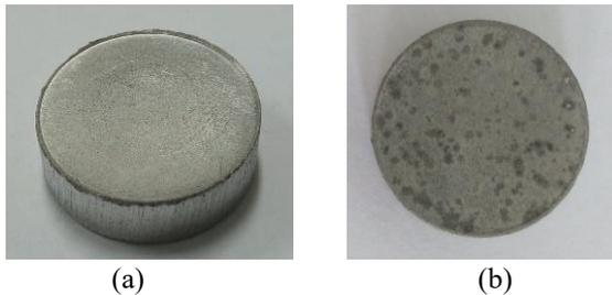
**Figure 3.** Composite sample for S4 with 5% graphite, (a) Green compact after compaction, (b). Sintered compact after sintered
